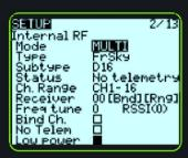
Frequency tuning. Certain protocols require tuning for optimal performance. In some cases, tuning is required in order for the protocol to bind. Frequency Tuning is specific to each MULTI-Module, and is due to very small variations in the RF components.
