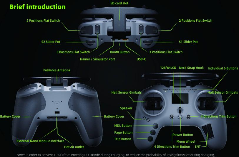
Note: In order to prevent T-PRO from entering DFU mode during charging, to reduce the probability of losing firmware during charging, T-PRO is the first radio that has a separate BOOTO button. When the radio is shut down, press and hold the BOOTO button, connect the USB cable, the system will enter DFU mode.
