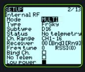
Status: Display the status of the multi-protocol module. (Normally it shows the firmware version of the multi-protocol module)
