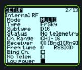
The default value of Freqtune is "0". If the receiver does not bind, we can change the value to either +30 or -30 and try to bind again. If binding is still unsuccessful, continue to try higher and lower values in steps of plus or minus 30 until the bind succeeds
